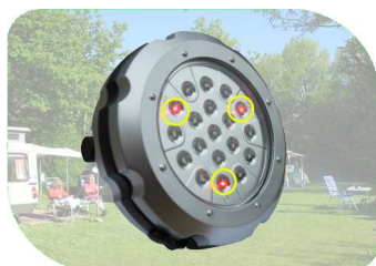
3 red warning light LEDs
